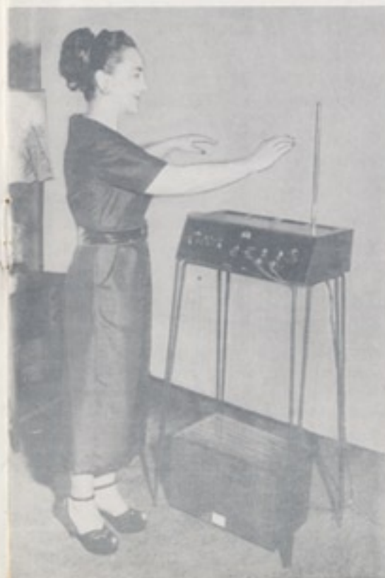
This is the position the performer assumes when playing the Theremin. Notice that the performer is not in physical contact with any part of the instrument.
