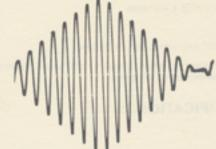
OUTPUT: LINEAR CONTROL MODE. IN-PUT IS 1 kHz. SINE WAVE . FIXED CON-TROL VOLTAGE = 3.
