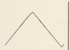
50 Hz TRIANGULAR WAVE 6 VOLTS PEAK-TO-PEAK, APPLIED TO CONTROL INPUT.
