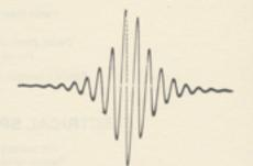
OUTPUT: EXPONENTIAL CONTROL MODE, INPUT IS 1 kHz. SINE WAVE. FIXED CONTROL VOLTAGE = 3.
