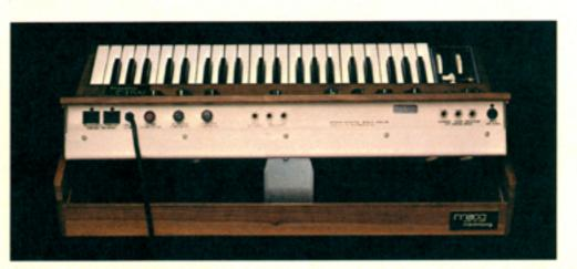
The accessory panel lets you add four different optional accessories to your Minimoog. Free your hands from the volume, pitch and filter controls with the optional Footpedal. Do it live with the Ribbon Controller for sliding, sweeping, soaring sounds. Or create a third hand for random and repetitive patterns with the Sample & Hold accessory. For the truly innovative drummer there's the Percussion Controller. The harder you hit it, the higher the pitch.
