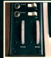
The Minimoog's unique left hand controllers let you really get inside. Grab the Pitch Wheel and bend your notes like a guitarist bends his strings. Roll the Modulation Wheel forward to bring in everything from vibrato to space effects. Flip a switch and rip up the keyboard with glide. Hit decay for sustain in legato passages. Or plug in the optional Footswitch to control glide and decay for the finished touch in performance control.
